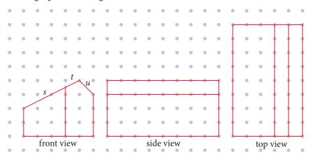
The distance between pairs of vertical or horizontal dots represents 5 ft. The house will be built in two sections and then transported to the building site for assembly. Highway traffic rules limit the width of each section to 15 ft or less. The centre wall will be located 15 ft from the left front wall. It will be doubly thick, so that each half of the house will have four walls during transport.
