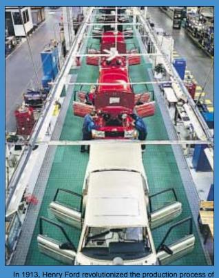
a car by pioneering mass-production manufacturing, a production system in which a conveyor belt brings each car to the workers, and each individual worker performs a single task along the production line. Even today, cars are built using this system, as shown in this photo of workers along a computerized automobile assembly line.
