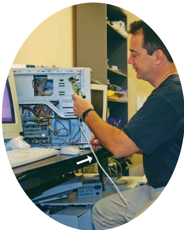
Figure 1.11 Static electric charges can damage sensitive electric equipment like computers. The arrow points to a special ground wire often worn by computer technicians to get rid of static electricity.
