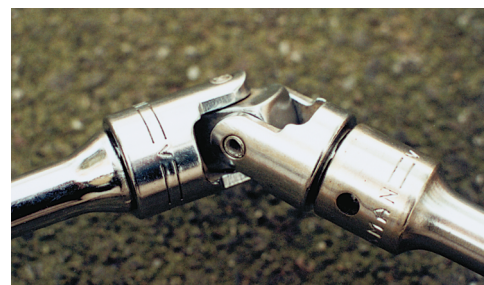
Photo 4.6 Universal joints, easily seen on the drive shafts of rear-wheel-drive cars and trucks, allow rotational motion to be transferred between two non-collinear shafts.
