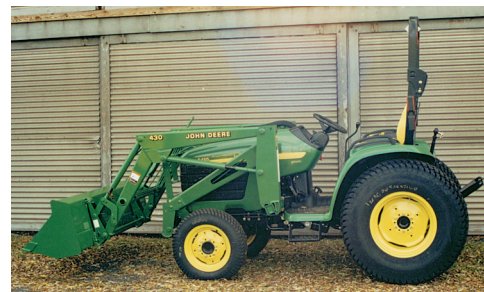
Photo 4.1 A free-body diagram of the tractor shown would include all of the external forces acting on the tractor: the weight of the tractor, the weight of the load in the bucket, and the forces exerted by the ground on the tires.
