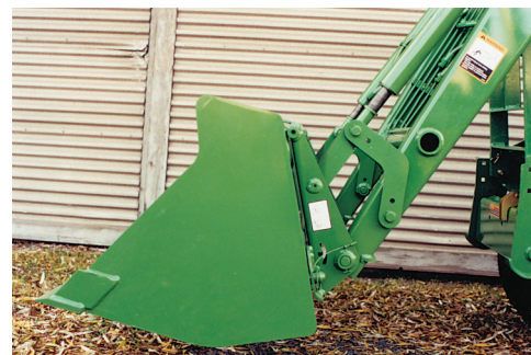
Photo 4.2 In chap. 6, we will discuss how to determine the internal forces in structures made of several connected pieces, such as the forces in the members that support the bucket of the tractor of Photo 4.1.
