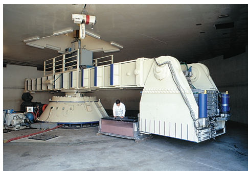
Photo 12.3 The path of specimen being tested in a centrifuge is a horizontal circle. The forces acting on the specimen and its acceleration may be resolved into radial and transverse components with r = \text{constant} .
