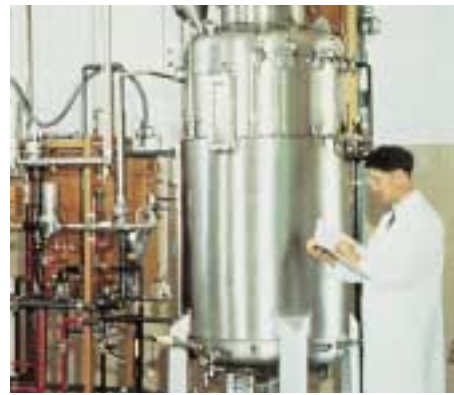
(a) Microbes as synthesizers. A large complex fermentor manufactures drugs and enzymes using microbial metabolism.
