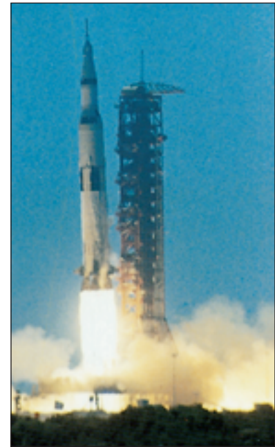
Apollo 11 lifts off its pad to begin the first human visit to the moon. The spacecraft's final speed was 10.8 km/s, which is equivalent to 6.7 mi/s. Conservation of linear momentum underlies rocket propulsion.
