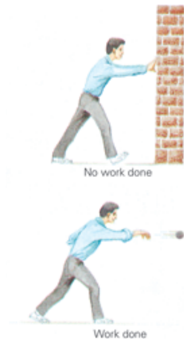
FIGURE 3-1 Work is done by a force when the object it acts on moves while the force is applied. No work is done by pushing against a stationary wall. Work is done when throwing a ball because the ball moves while being pushed during the throw.
