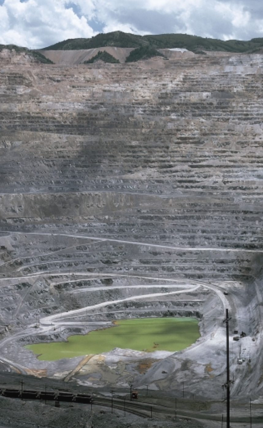
FIGURE 11.10 The world's largest open-pit mine is Bingham Canyon, near Salt Lake City, UT. More than 5 billion tons of copper ore and waste material have been removed since 1906 to create a hole 800 m (2,640 ft) deep and nearly 4 km (2.5 mi) wide at the top.
