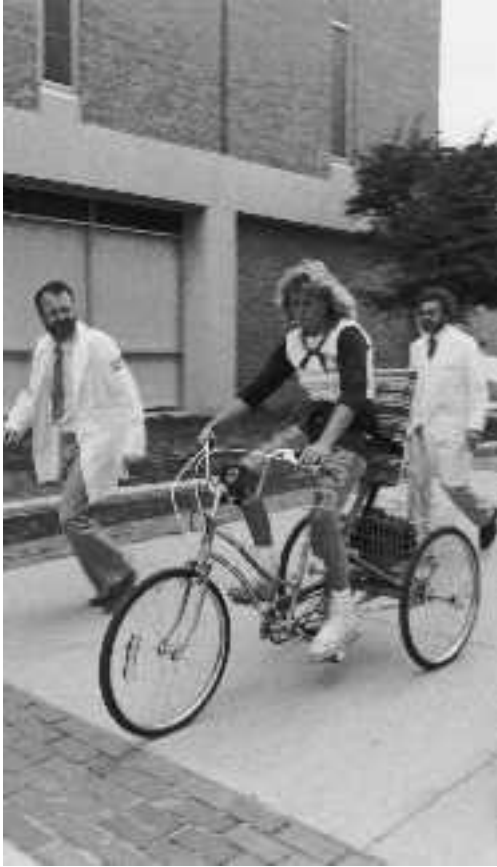
Figure 1-4 This young woman suffered three transections of her spinal cord in an automobile accident. She is shown pedaling a cycle around the Wright State University campus by means of computer-controlled, functional electrical stimulation of her paralyzed leg muscles. Фото: Courtesy of Roger Glaser.
