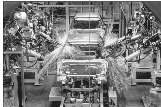
Figure 1.13 Computerized robots weld a 1994 GM vehicle in Shreveport, LA. (© Charles O'Rear/CORBIS.)
