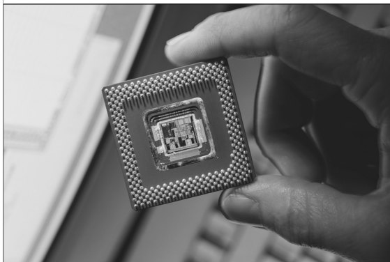
Figure 1.12 Modern microprocessors have a multitude of outlets, as indicated on this picture of Intel's Pentium II microprocessor. (© Don Mason/CORBIS.)
