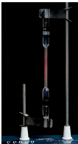
Color emitted by hydrogen atoms in a discharge tube. The color observed results from the combination of the colors emitted in the visible spectrum.
