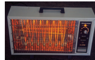
The red glow of an electric heater is an example of blackbody radiation.
