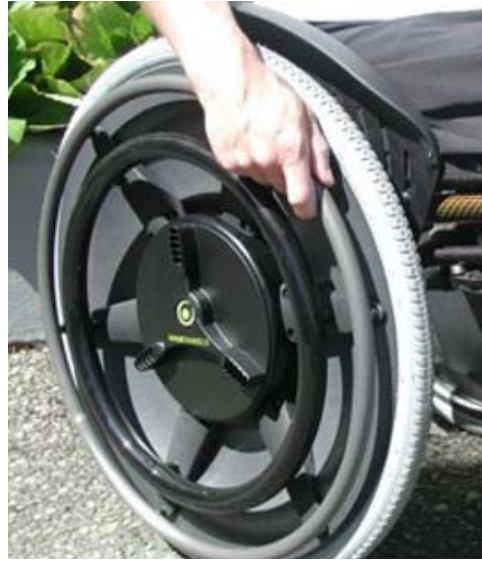
Figure 2: Pushing on the hand rim and details of a MAGICWheels 2-gear wheel
