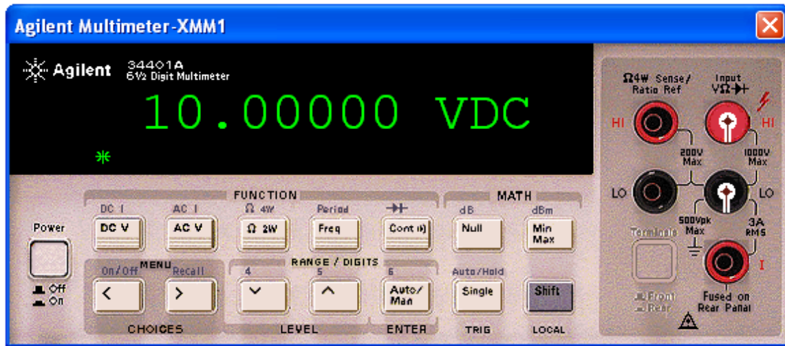
Figure 46 DC Voltage Measurement with an Agilent Multimeter
