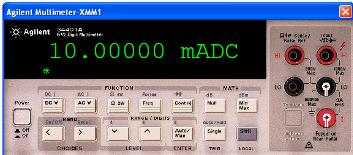
Figure 52 DC Current Measurement with an Agilent Multimeter
