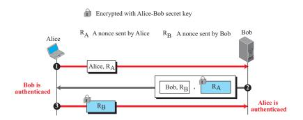
**P31-27.** The following shows the new diagram. Two nonces and two keys are used to achieve bidirectional authentication.
