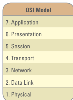
FIGURE B5.10 Open System Interconnection Model
