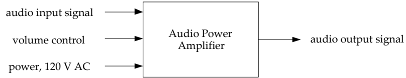
Figure 5.2 Level 0 audio power amplifier functionality.
