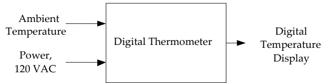
Figure 5.9 Level 0 digital thermometer functionality.
