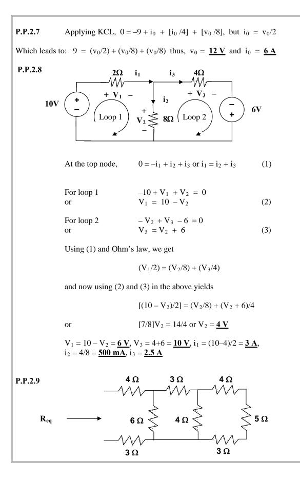
Combining the 4 ohm, 5 ohm, and 30hm resistors in series gives 4+3+5 = 12. But, 4 in parallel with 12 produces [4x12]/[4+12] = 48/16 = 30hm.
