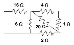
The 4 ohm and 1 ohm resistors can be combined into a 5 ohm resistor in parallel with a 20 ohm resistor. This will result in [5x20/(5+20)] = 4 ohms and the circuit shown below:
