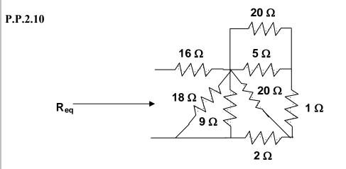
Combining the 9 ohm resistor and the 18 ohm resistor yields [9x18]/[9+18] = 6 ohms.
