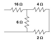
The 4 ohm and 2 ohm resistors are in series and can be replaced by a 6 ohm resistor. This gives a 6 ohm resistor in parallel with a 6 ohm resistor, [6x6/(6+6)] = 3 ohms. We now have a 3 ohm resistor in series with a 16 ohm resistor or 3 + 16 = 19 ohms. Therefore:
