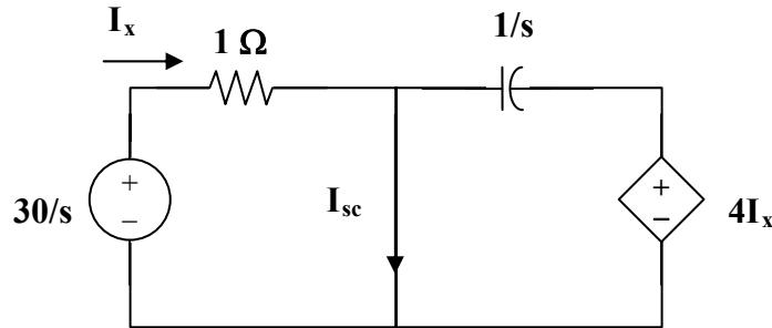
$$I_x = (30/s)/1 = 30/s \quad I_{sc} = 30/s + 4(30/s)/(1/s) = 30/s + 120 = (120s+30)/s = 120(s+0.25)/s$$
