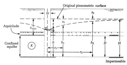
FIGURE 2-5 Geometry and symbols for a pumped well in a confined aquifer. (*Source:* H. Bouwer, 1978.)
