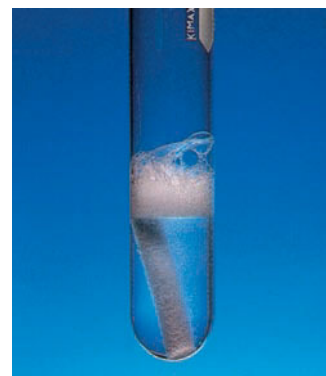
Figure 4.6 A piece of blackboard chalk, which is mostly \text{CaCO}_3 , reacts with hydrochloric acid to produce carbon dioxide gas.
