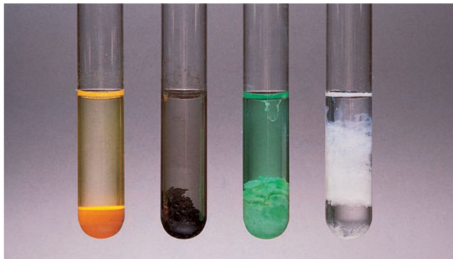
Figure 4.4 Appearance of several precipitates. From left to right: \text{CdS} , \text{PbS} , \text{Ni(OH)}_2 , \text{Al(OH)}_3 .
