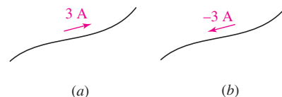
■ FIGURE 2.5 Two methods of representation for the exact same current.
