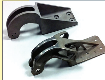
Lighter Load: A conventional hinge for the corner of a jet engine (top) could be replaced by the more intricate one at bottom, which is just as strong but weighs half as much. The new design, created by EADS, is made practical by three-dimensional printing technology.
