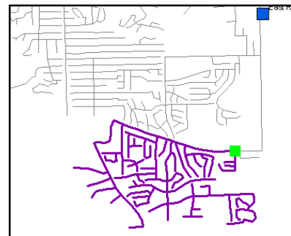
Fig. 9.12. Trace Downstream could find the service area disrupted by a broken pipe.
