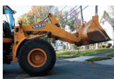
Photo 4.2 In Chap. 6, we will discuss how to determine the internal forces in structures made of several connected pieces, such as the forces in the members that support the bucket of the tractor of Photo 4.1.
