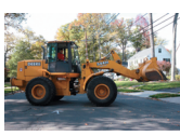
Photo 4.1 A free-body diagram of the tractor shown would include all of the external forces acting on the tractor: the weight of the tractor, the weight of the load in the bucket, and the forces exerted by the ground on the tires.
