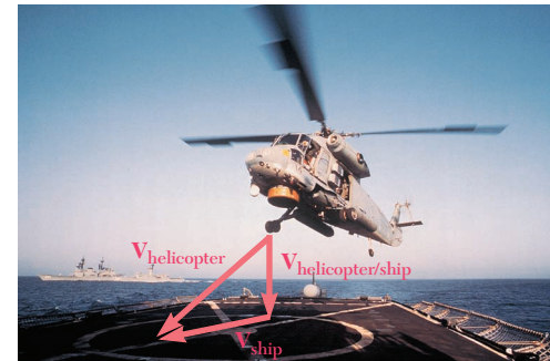
Photo 11.4 The pilot of a helicopter landing on a moving carrier must take into account the relative motion of the ship.
