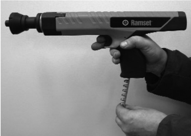
Fig. 17.12B Step 2: Insert the power load
