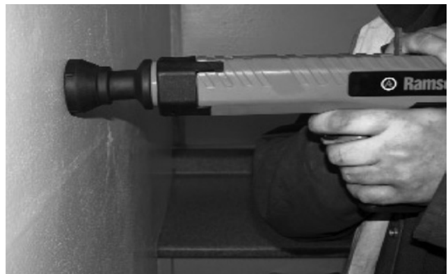
Fig. 17.12E Step 5: Fire the tool
