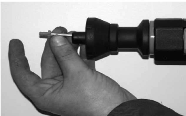
Fig. 17.12C Step 3: Select and insert the fastener
