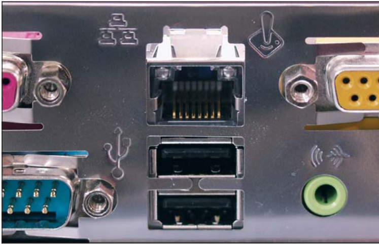
• Figure 4.21 RJ-45 port above two USB ports
