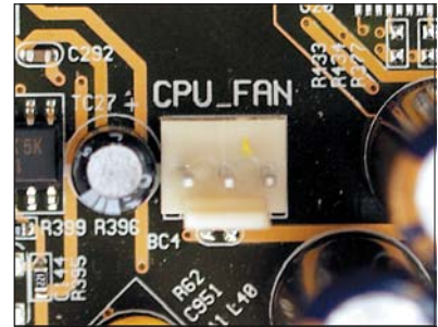
• Figure 4.3 Power connector for the CPU fan
