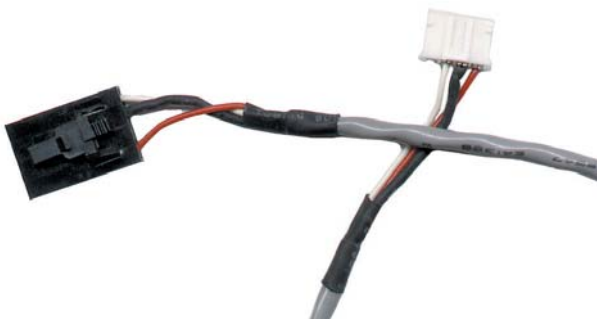
• Figure 4.23 Special audio cable for a CD-ROM drive
