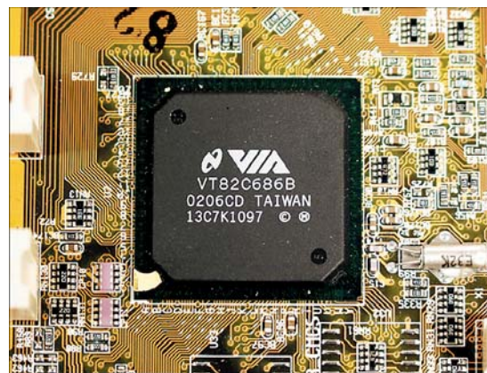
• Figure 4.9 A VIA Southbridge chip on a motherboard
