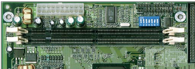
• Figure 4.4 Memory slots on an ATX motherboard
