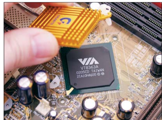
• Figure 4.8 A VIA Northbridge chip on a motherboard. The tech is holding its heat sink.
