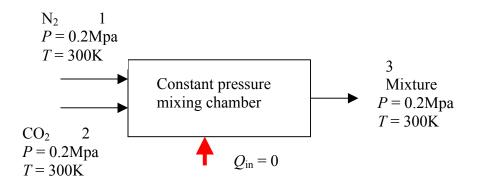
Take the time to apply the steady-flow conservation of energy and mass to show that the temperature of the mixture at state 3 is 300 K.
