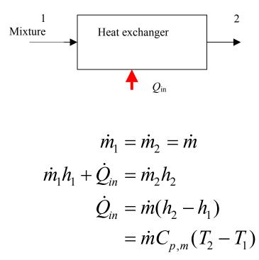
The heat transfer per unit mass flow is
