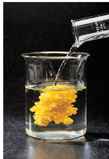
Figure 4.6 The reaction of Pb(NO 3 ) 2 and NaI. When aqueous solutions of these ionic compounds are mixed, the yellow solid PbI 2 forms.
