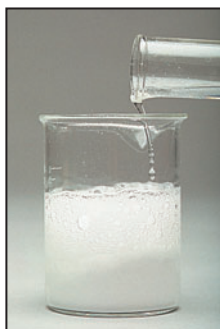
Figure 4.9 An acid-base reaction that forms a gaseous product. Carbonates and hydrogen carbonates react with acids to form gaseous \text{CO}_2 and \text{H}_2\text{O} . Here, dilute acetic acid solution (vinegar) is added to sodium hydrogen carbonate (baking soda) solution, and bubbles of \text{CO}_2 gas form. (Note that the net ionic equation includes acetic acid because it is a weak acid and does not dissociate into ions to an appreciable extent.)
