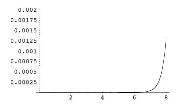
This looks very good. Although the error clearly grows exponentially, it less than 0.0015 at t = 8 (years, maybe?). We say years because at t = 8 the approximate solution vector is over 3.6 x  $10^{12}$  units long. (The length calculation uses the Euclidean norm.)
