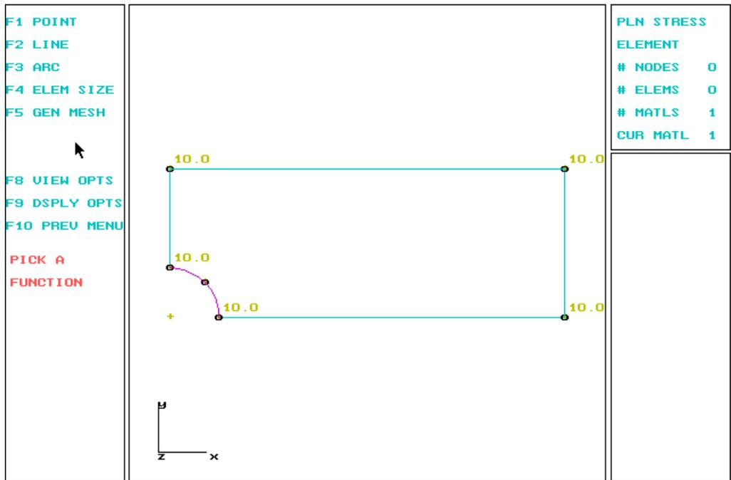
The next stage is to generate a first mesh for analyzing the model. The principle behind the mesh generation in FEPCIP is to map a grid array of squares into the actual geometry. Please read the section in the user's guide describing the mesh generation procedure before continuing this tutorial.
