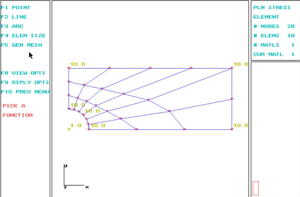
The next step is to apply the displacement restraints to satisfy symmetry and the loads. Symmetry requires that all nodes lying on a plane of symmetry must remain on the plane after loading. Therefore all motion that would take the node off the plane must be restricted.
