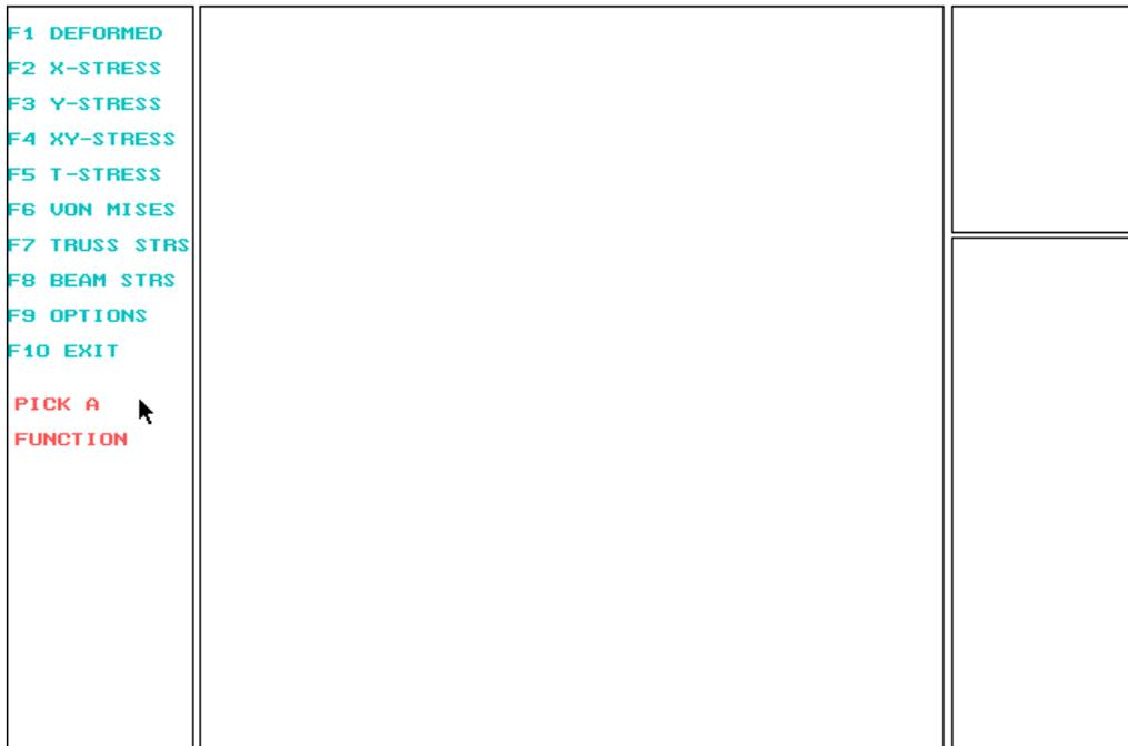
In output processing, the deformed shape and element stresses may be examined. The deformed shape provides opportunity to determine if the shape is realistic based on engineering intuition and to check that symmetry boundary conditions and loads have been realistically applied.
