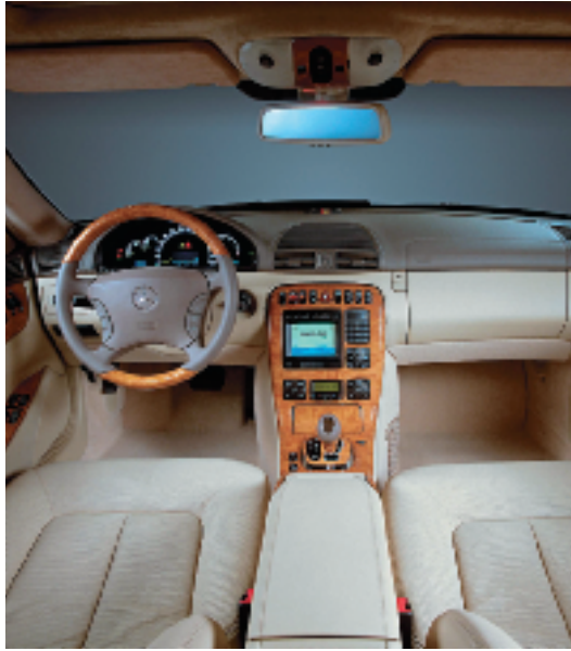
Interactivity. A dashboard computer allows drivers to request information about their car's operation, geographic location, and nearby services.
