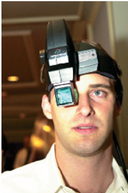
(Left) Micro Vision's Retinal Scanning Display records what the user is seeing and sends the data to a mode worn on the user's belt. (Right) The HandsFreeMobile e-Belt wearable computer.
