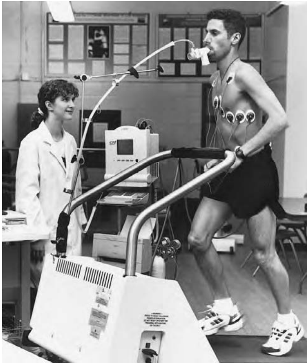
Figure 3.18 \dot{V}O_{2max} can be estimated accurately from performance time on the treadmill if the subject is taken to a “true max” and does not hold onto the treadmill bar.
