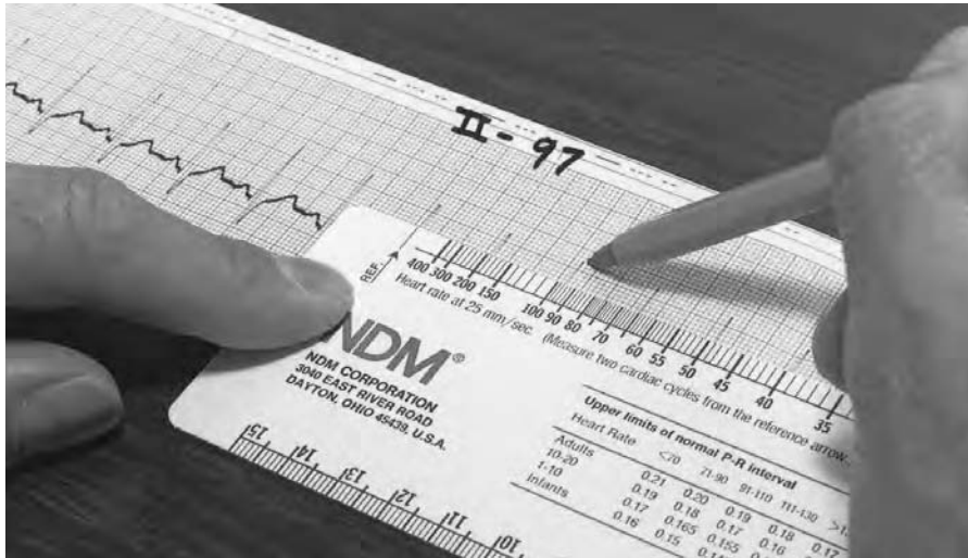
Figure 3.7 The heart rate can be determined from an ECG recording by using a heart rate ruler. With this particular ruler, heart rate is determined by reading the ruler after counting two heart rate cycles to the right of the reference arrow.
