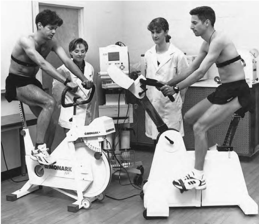
Figure 3.12 Mechanically braked cycle ergometers such as the Monark model pictured here have a front flywheel braked by a belt running around the rim attached to a weighted pendulum. The workload is adjusted by tightening or loosening the brake belt. The pedaling rate has to be maintained by the exerciser in time to a metronome. Good mechanically braked models cost between $750 and $1,000. The electronically braked ergometer uses an electromagnetic braking force to adjust the workload. The resistance is variable in relation to the pedaling rate, so that a constant work output in watts is maintained. However, electronically braked ergometers cost over $2,500.
