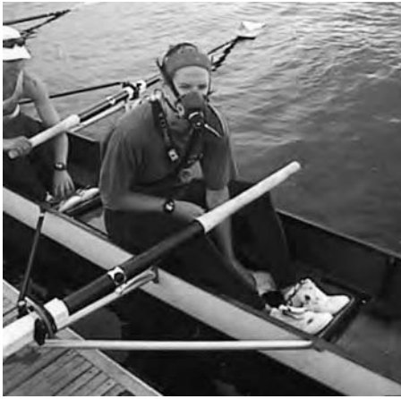
Figure 1.1 The K4b2 (COSMED Ltd., Rome, Italy) is a fully portable breath-by-breath pulmonary gas exchange system for measuring energy expenditure away from the lab.
