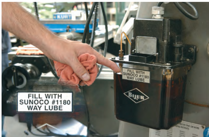
Figure 1-16 Be absolutely certain to add the right oil, especially on CNC equipment!
