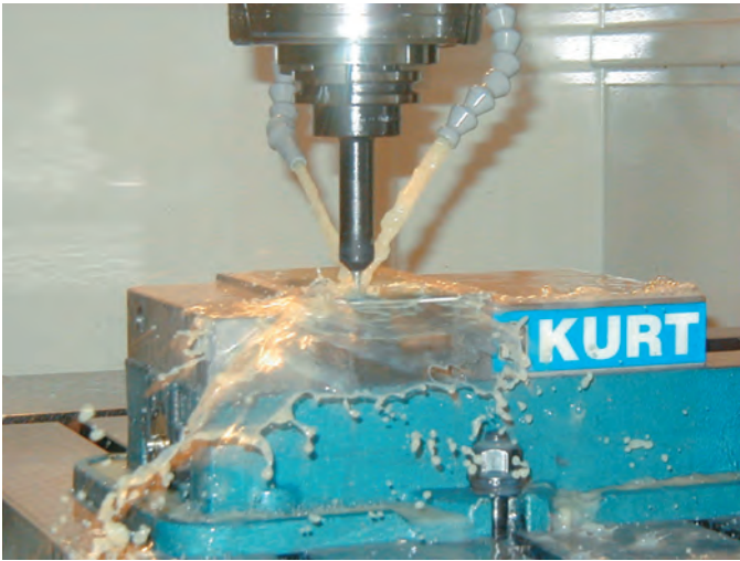
Figure 1-17 Synthetic coolants are highly designed shop chemicals that are mixed with water to make machining more efficient and safer.
