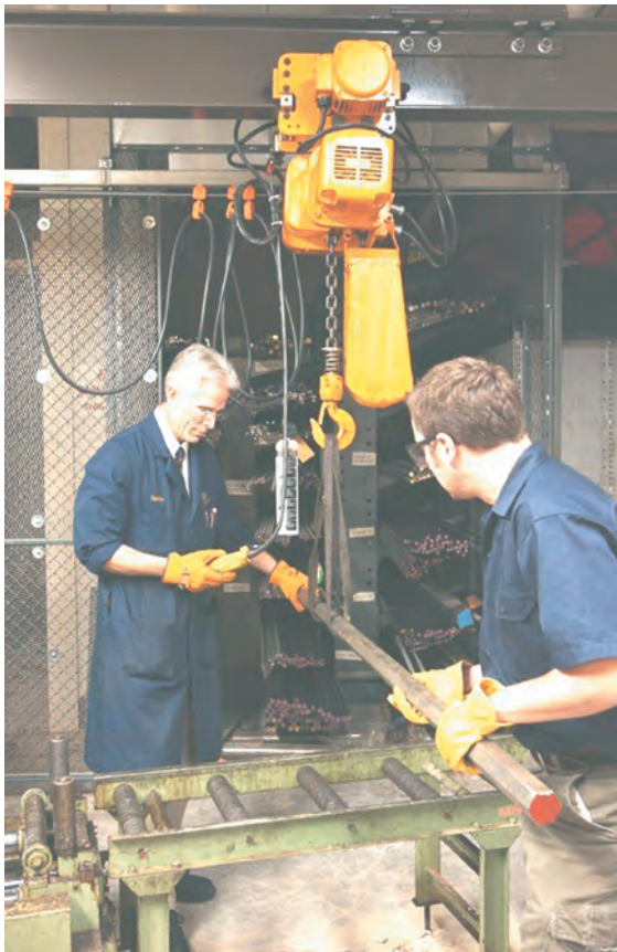
Figure 1-11 Use a crane and choker to haul heavy bars, while an assistant helps control the metal bar!
