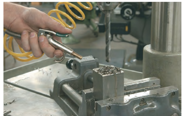
Figure 1-25 Compressed air is a good chip removal and cleanup tool when correctly used.
