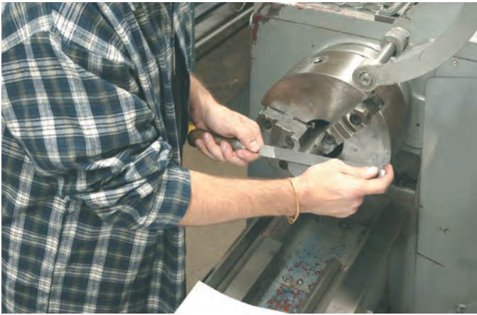
Figure 1-6 Jewelry is dangerous. It catches on machines and chips and conducts heat and electricity.
