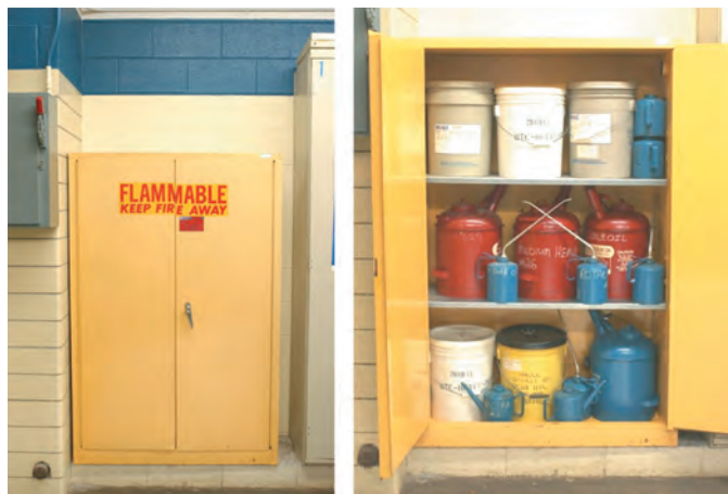
Figure 1-15 Specialized lubricants must be stored in fireproof surroundings and kept free from contamination.
