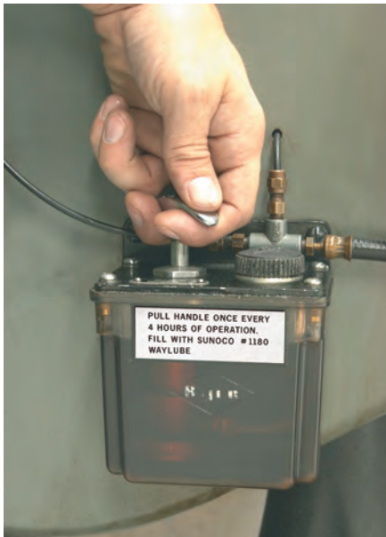
Figure 1-27 A one-shot central lubricator. Use at least once per half day or on the schedule set by your instructor.
