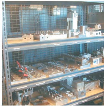
Figure 1-30 Machine accessories must be stored and transported correctly. Make sure they are on shelves made for heavy storage.
