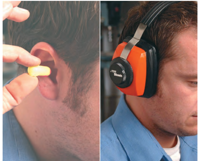
Figure 1-3 Machinists protect their hearing when shop noise is loud or high pitched.
