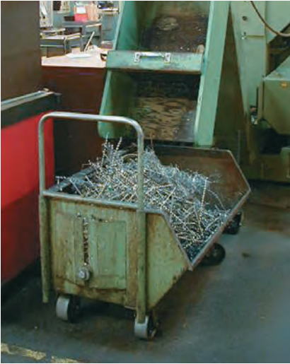
Figure 1-20 Chips can pile up quickly and must be removed from the machine.
