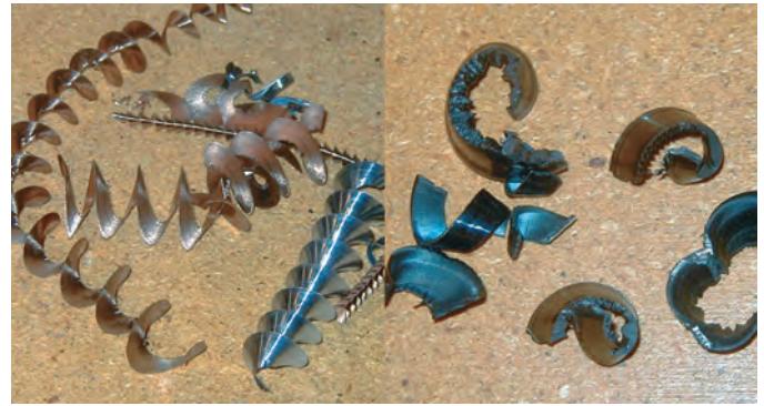
Figure 1-19 Long, stringy chips are strong razor wires that catch clothing and cut skin. All chips, even the safer "C" shapes on the right, can be dangerously hot.
