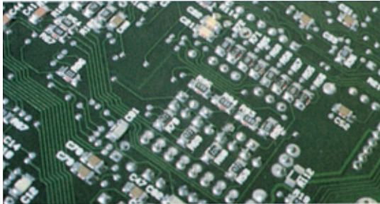
A comparison of conventional-mount and surface-mount technologies. (a) The photo shows both methods, and the drawing shows the conventional method. (b) Photo and drawing of a surface-mount technology ( SMT ) circuit board.
