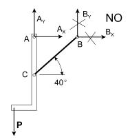
wrong to include member CB in the FBD, but the reaction at C must recognize that CB is two-force.
