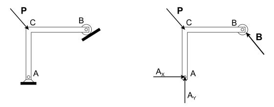
In the example above, force **A** has been entered as components in the positive x and y directions. Calculations will give a negative sign for  $A_x$ , showing that  $A_x$  in reality points in the negative x direction. If this happens, **DO NOT** go back and change the free-body diagram. Simply note in your solution that "positive force directions are as shown in the FBD", or show the force direction unambiguously in giving your answer.
