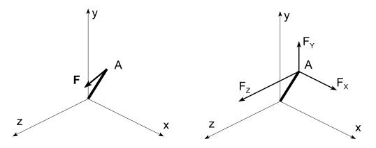
**3.** Forces must be labelled. Labelling is necessary to define your notation, so that the marker can understand the algebraic part of your solution. A FBD with the forces unlabelled is WRONG.
