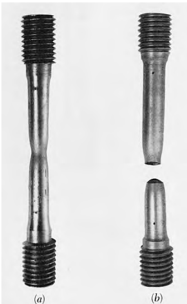
Photo 2.4 Ductile material tested specimens: (a) with cross-section necking, (b) ruptured.
