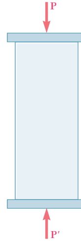
Fig. 2.46 Axial load applied by rigid plates.
