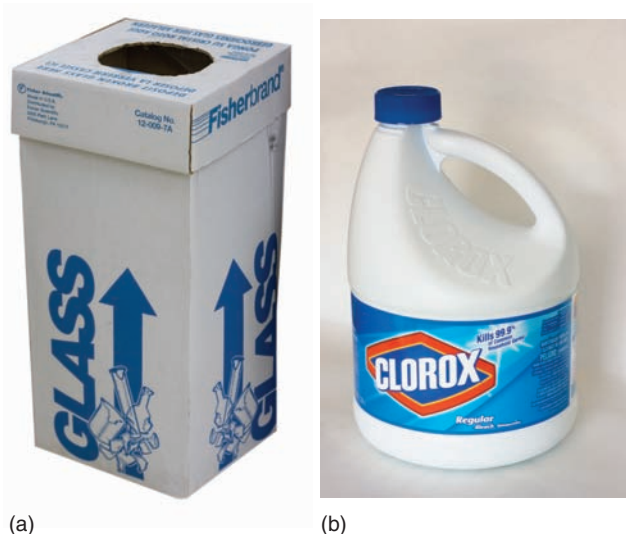
Figure 1-5 (a) Clean up broken glass with care and place in proper container; (b) Freshly prepared solutions of 10% household bleach may be used to sanitize the area or commercially available spill kits may be used.
