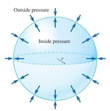
**Figure 9.S1** In a soap bubble, the air pressure inside is higher than the pressure outside.
