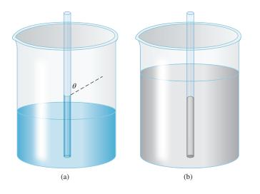
**Figure 9.S2** Capillary tube in (a) water and (b) mercury
