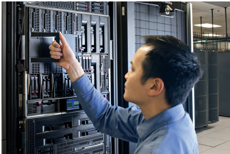
Figure 1.7 Blades are full PCs in a narrow box suitable for side-by-side installation.
