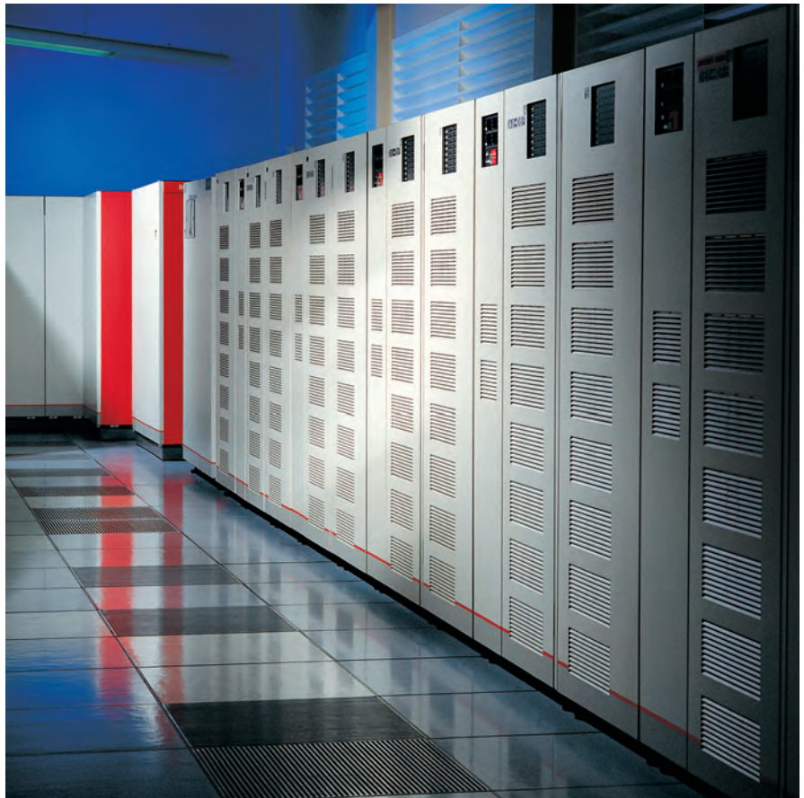
Figure 1.8 Mainframe computers are often housed alone in special rooms, away from their users.
