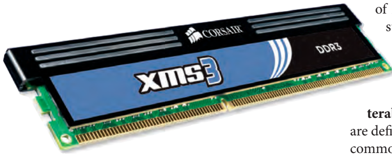
Figure 1.18 RAM for a PC comes in modules ready to be installed into the motherboard.
