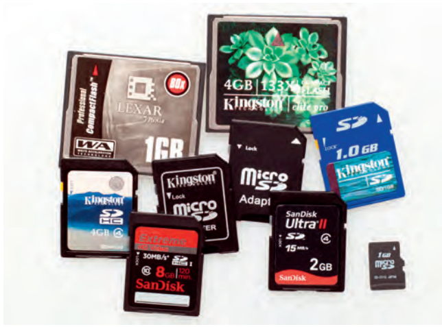
Figure 1.20 Solid state drives have no moving parts; perfect for small devices with limited power.
