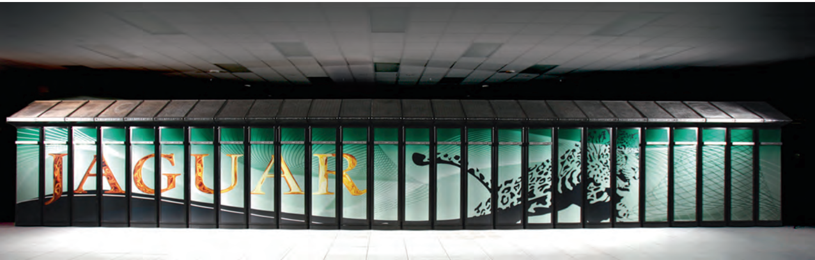
Figure 1.9 Supercomputers like Cray’s XT5 Jaguar are massive machines, integrating hundreds of thousands of smaller processors together.
