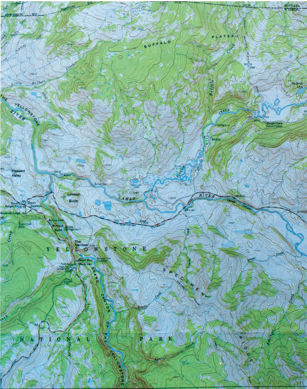
FIGURE B.4 Representative section of standard topographic map: a portion of Yellowstone National Park. Note the closely spaced contours along the Grand Canyon of the Yellowstone and edges of plateaus, the shapes of contours that cross streams, the closed contours around hills (for example, Junction Butte), and the swampy flat area (along Slough Creek).
